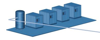
While everything is optimized for cost saving in production, the compressors in most compressed air stations are controlled according to fixed sequences. Manual pressure switches and simple electronic controllers are switched the compressors. The pressure in the network is significantly higher than required in production. This leads to high energy costs and excessive wear on the compressors due to frequent changes of load..
