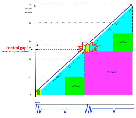
The result is, the VSD compressor falls below its minimum delivery and the pressure rises to Pmax, where the just switched on compressor will switch off again. Consequently the VSD compressor rises to full power from standstill or idle, but is still not sufficient and the just switched off compressor will again switch on.
