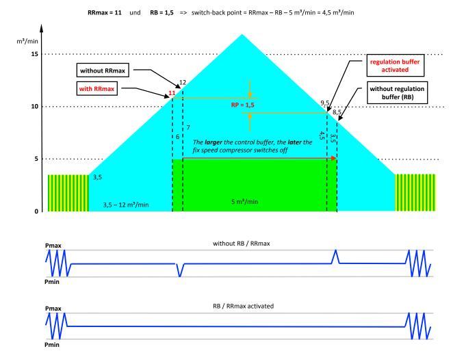
When using the control parameters **RRmax** and **RB**, the fix speed compressors are switched dynamically - without touching Pmin and Pmax!
