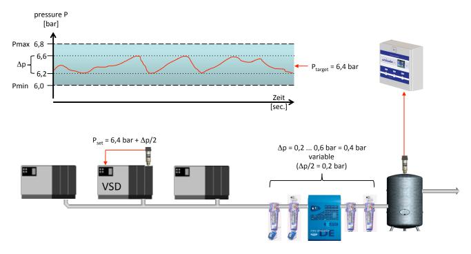
The Airleader control parameters **Pmax – Pmin**, determining the control pressure range, **must be set to a larger range** (+  $\Delta$ P). This works mostly- **but not in terms of an energy-efficient operation.**
