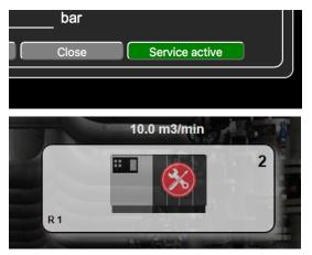
The grey "Activate Service" button changes to "Service active" and turns green. Another click on this button ends the maintenance mode and the compressor can be immediately re-selected by the Airleader.
