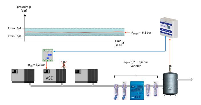
The Airleader control pressure is a 4 - 20 mA signal at the analogue output AO of the RS 485 connection module within the compressor. The analogue signal can be scaled according to the pressure range of the compressors pressure transducer via the menu. By default 4 .. 20 mA = 0 .. 16 bar are pre-set.
