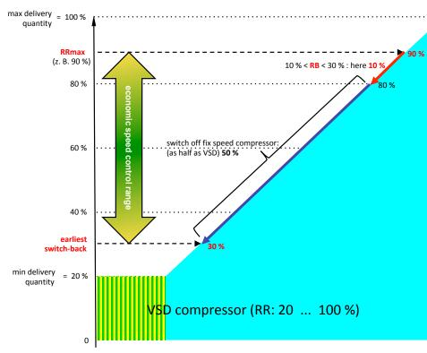
Airleader observes a certain time the speed falling below the limit and then switches off a compressor, so that the VSD compressor can regulate to higher, more economical speed. (Trend: consumption continues to decrease).
