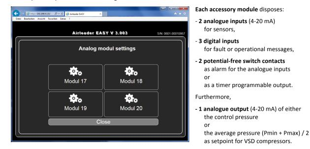
Here, for example, with one accessory module can be monitored the room temperature and the filter differential pressure, as well as a dryer fault message, a condensate failure and an operating message (fan, pump, etc.).
